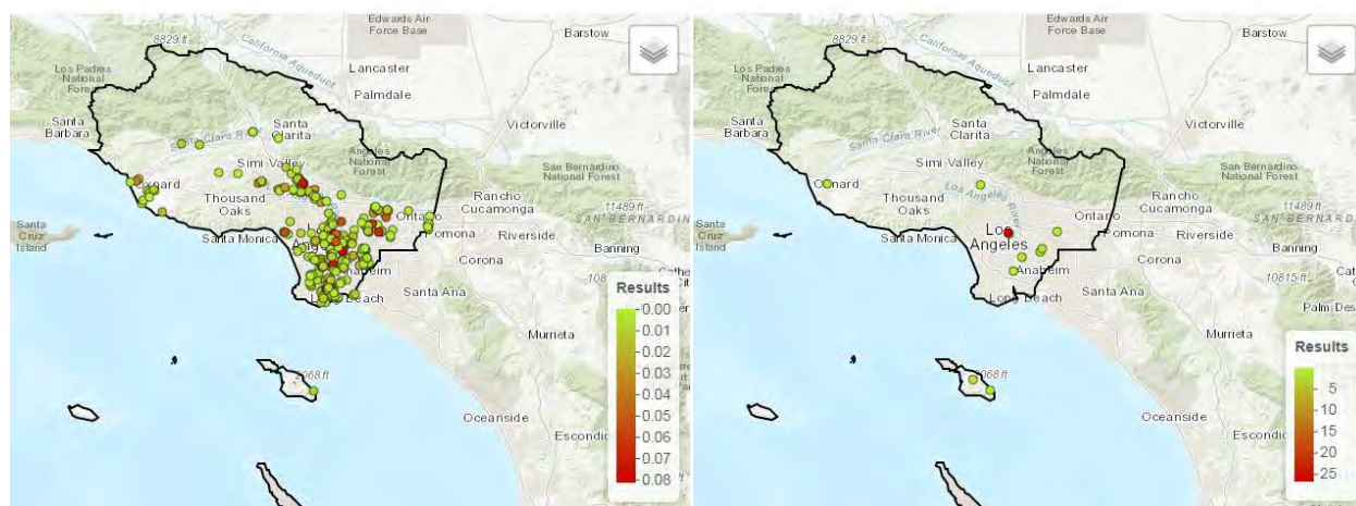
FIGURE 3-1 Median lead concentrations at sites in California Water Board, Los Angeles Region, from monitoring from the past 5 years, with results less than (left) and greater than (right) the benchmark of 82 µg/L.
