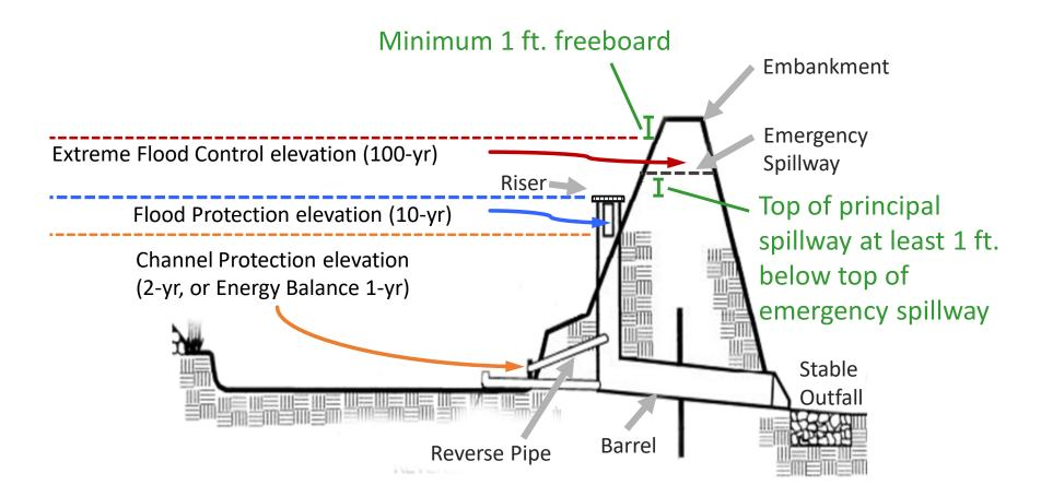
Water quantity compliance on approved plan/installed pond achieved via size of riser pipe, size of riser orifice(s), size of outflow pipes, and barrel size. Pipe materials/specs should be verified in accordance with approved plan
