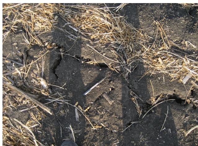
Figure 3: Cracks in clay soils with high shrink-swell capacity.
