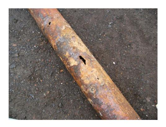
Stand pipe from pump station downstream of brewery, due to low pH, high temp & HS
