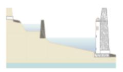
An extended detention basin is a stormwater management facility that temporarily stores and attenuates stormwater runoff. In addition, extended detention basins provide pollutant treatment for runoff from the Water Quality Design Storm through settling. When designed in accordance with this chapter, the total suspended solids (TSS) removal rate is 40 - 60%, depending on the duration of runoff detention.
