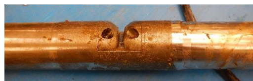
Probe contaminated by sediments and biofouling.
