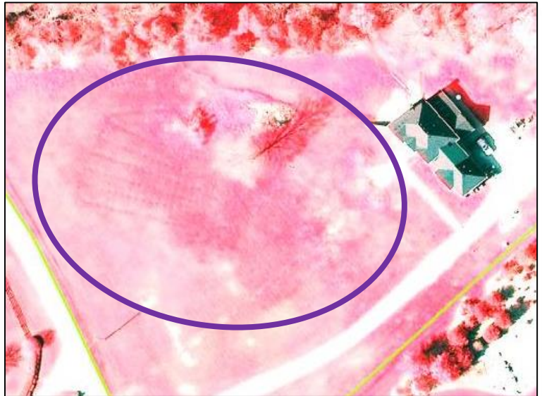
This image shows the lines of a septic field.
