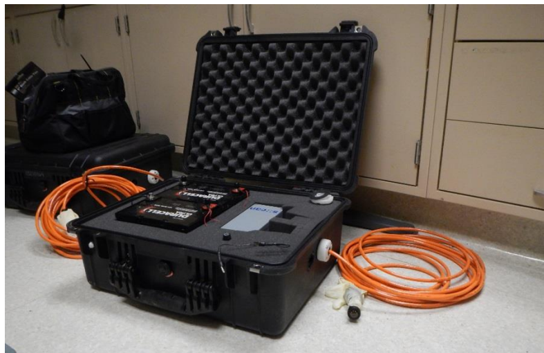
Batteries and S::CAN electronics in waterproof case with marine grade connectors.
